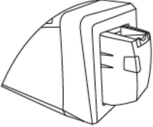
A line drawing of the card hopper assembly. The cover is shown closed, and the lever is now in an upward position, ready for printing.                                                                                                                                                                                                    |
