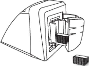
A line drawing of the card hopper assembly. A card is shown being inserted into the tray. Below the hopper, a separate card with a magnetic stripe is shown, indicating the correct orientation for loading. |
