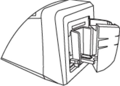
A line drawing of the card hopper assembly. A lever on the right side is shown in a downward position, locking the card tray into place.                                                                                                                                                                                                   |
